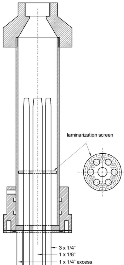
Figure 2: Example sketch for an isokinetic flow splitter
