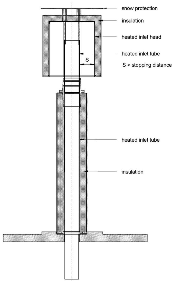
Figure 1: sketch of a whole air inlet
